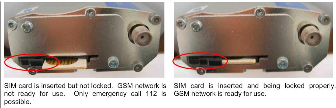
Figure 11: SIM card lock feature
